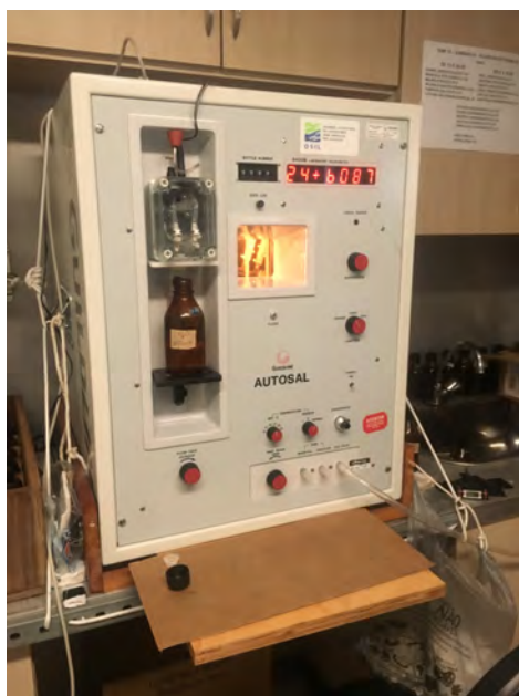
Figure 5.3.1: Autosal Guildline 8400B bench salinometer used for on board salinity analysis.
