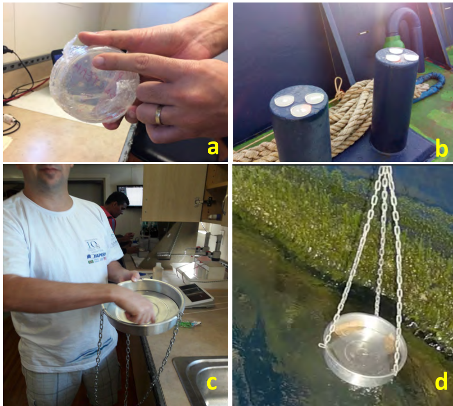
Fig. 37: Instruments for microbiology sampling, in the atmosphere (a,b) and in the ocean's critical layer (c,d). The samples were collected by C. Teixeira and will be analyzed at LABOMAR/UFC.
