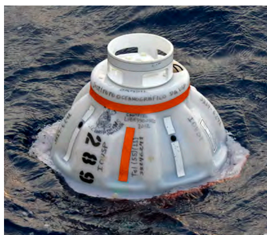
Fig. 10: C-PIES SN289 recovered from site AA. Relunched on site BB.
