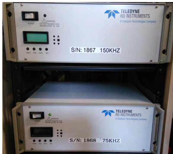
Figure 20. Deck unit controlling each VMADCP located in the main lab.
