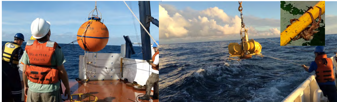
Fig. 8: Pictures taken during the operations with the ADCP (left) and the BPR (right). The insert shows a little crab that took a ride from the bottom to the surface, on the BPR.
